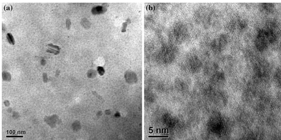
of fine precipitates possibly  $\eta'$  or a transition phase from the GP-zones along with sparsely distributed coarse dispersoids called E-phase [15]. Our EDS analysis confirmed that the E-phase dispersoids are enriched in chromium and these have been shown not to dissolve during solutionizing [15]. The fine precipitates are generally accepted to be the
