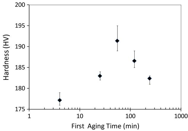
**Fig. 5** Effect of time of first aging at 121 °C on peak hardness of second aging at 177 °C of AA7075 alloy. Note 55 min of first aging has the highest peak hardness after second aging
