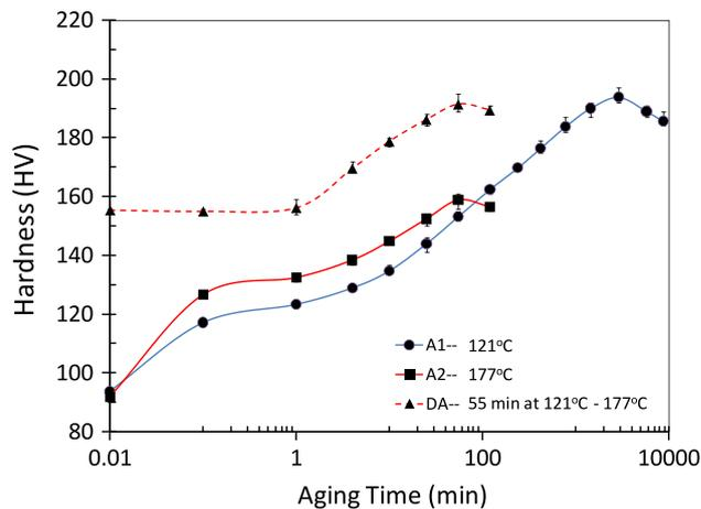
**Fig. 3** Effect of single and double aging on hardness of AA7075 alloy. Note peak hardness of the DA is comparable to A1
