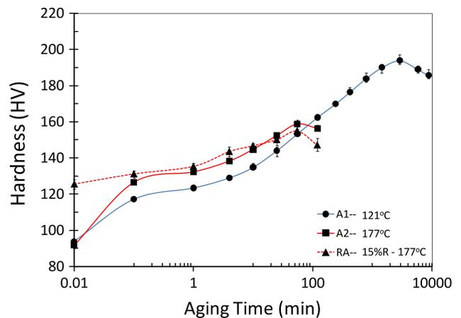
**Fig. 7** Effect of rolling prior to single aging of AA7075 alloy. Note the decrease in peak hardness in RA
