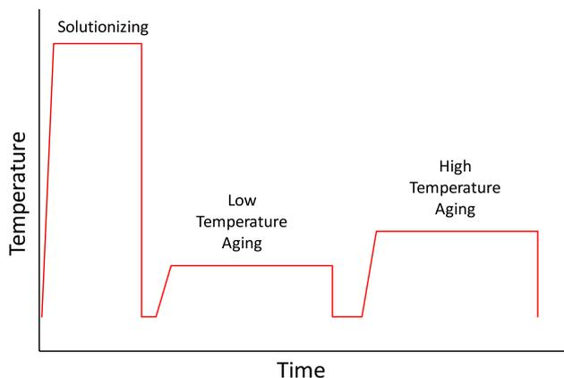
**Fig. 1** Heat treatment profile of double aging (DA)
