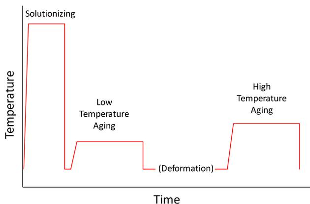
**Fig. 2** Heat treatment profile of thermomechanical double aging (TMDA)
