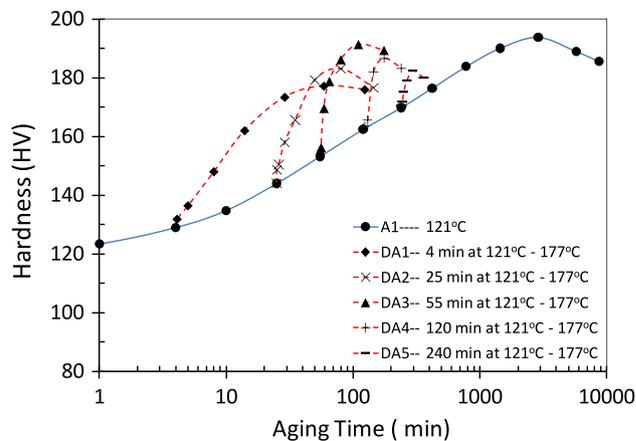
**Fig. 4** Effect of time of first aging on double aging of AA7075 Alloy. Note the peak hardness of DA curves change with time
