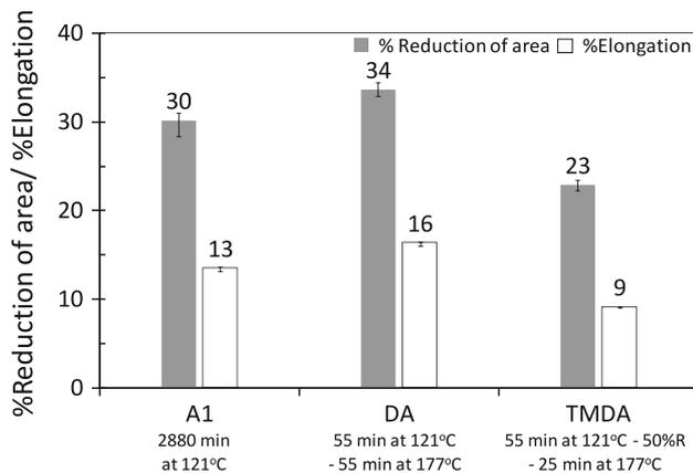
**Fig. 15** Ductility of AA7075 alloy after A1, DA, and TMDA2 treatments
