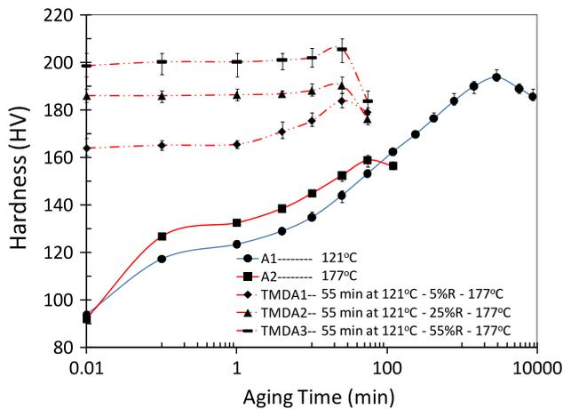
**Fig. 6** Effect of TMDA on hardness of AA7075 alloy. Note the peak hardness of TMDA3 is higher than A1 and the line curve stays flat initially indicating simultaneous recovery and precipitation
