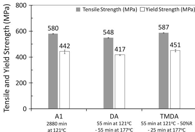
**Fig. 14** Yield and tensile strength of AA7075 alloy after A1, DA, and TMDA2 treatments
