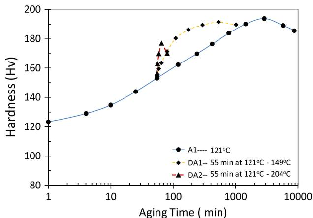
**Fig. 12** Effect of second aging temperature on DA treatment of AA7075 alloy. Note the peak hardness of DA2 is lower due to the dissolution of the GP-zones
