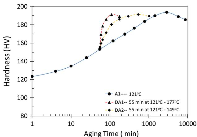
**Fig. 11** Effect of second aging temperature on DA treatment of AA7075 alloy. Note the peak hardness of both DA treatments are the same
