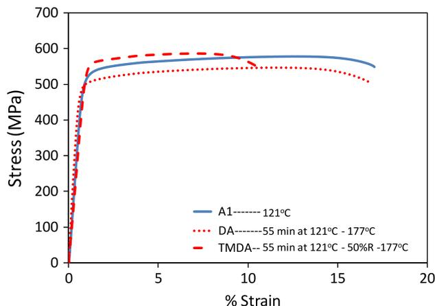
**Fig. 13** Engineering stress–strain curves for AA7075 alloy after A1, DA, and TMDA2 treatments
